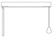
Control wand on the left, cord on the right "KD"
